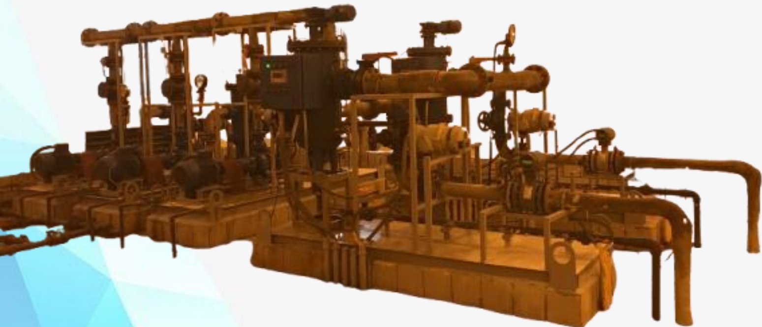
Figure 06: Maintaining Chlorination Systems in Power Plants: A Critical Measure Against Biofouling. The chlorine-generating section of a power plant plays a vital role in preventing the growth of marine biota, which can lead to biofouling. Biofouling not only impairs equipment functionality but also significantly reduces plant efficiency. Effective chlorination is essential to mitigate these risks and ensure optimal operational performance. – Aravinda Ravibhanu © 2017
